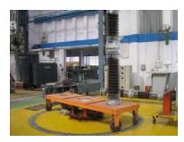
Net/cage provided for HV test room
