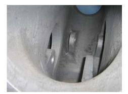
Assembly of closing/tripping mechanism
