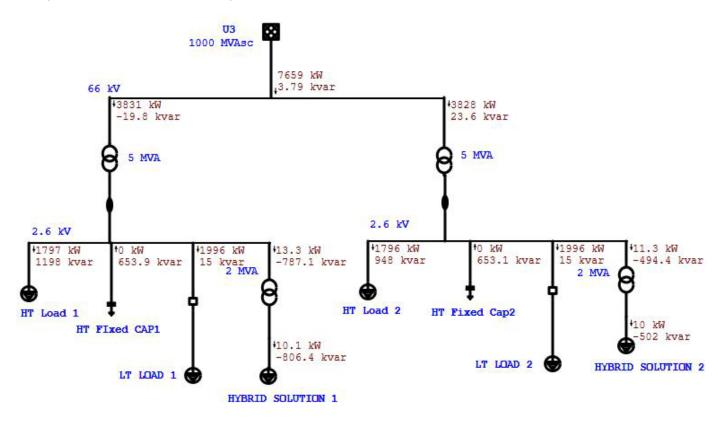
For the plant under consideration, the total solution will cost around Rs. 200Lacs and the payback will be around 2 years. Improvement in internal power quality and reduction in distribution loss will be additional benefits.
